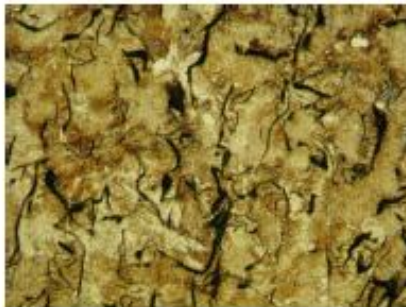
Brake surface sample 6616G at 250x mag 2% Nital Etch
