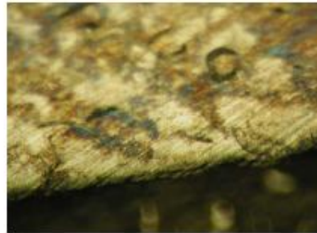
Brake surface sample 6616G at 250x mag 2% Nital Etch
