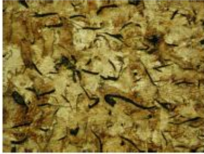
The microstructure of the core section of sample 6616G exhibited a characteristic pearlitic graphite flake cast iron structure.
